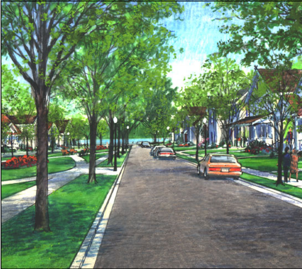
Figure 5.23: Simple treatments such as this concrete walk and tree-planting strip (or concrete walks with grassed tree pits for narrower right-of-way) are appropriate to improve residential streetscapes and vehicular streets such as Concord Avenue and Vandever. Trees and well-maintained walks can make a tremendous difference in perceptions about the quality of a neighborhood.
